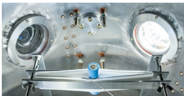
An Accelerated Rate Calorimeter from Akkurate for testing batteries. It can be used for measuring heat capacity, thermal stability of the cell or heat generation during usage.
