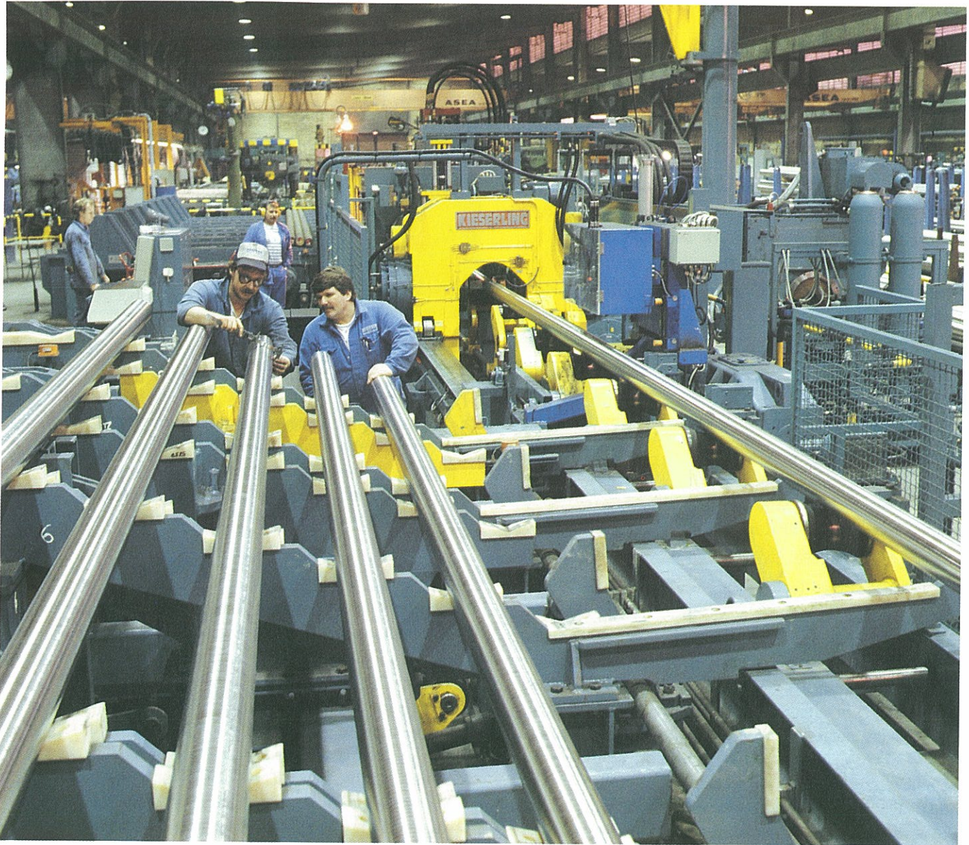
A new bar-peeling machine has been installed in the billet-conditioning department at Sandviken. It boosts productivity and raises the quality of bars and tube hollows.
