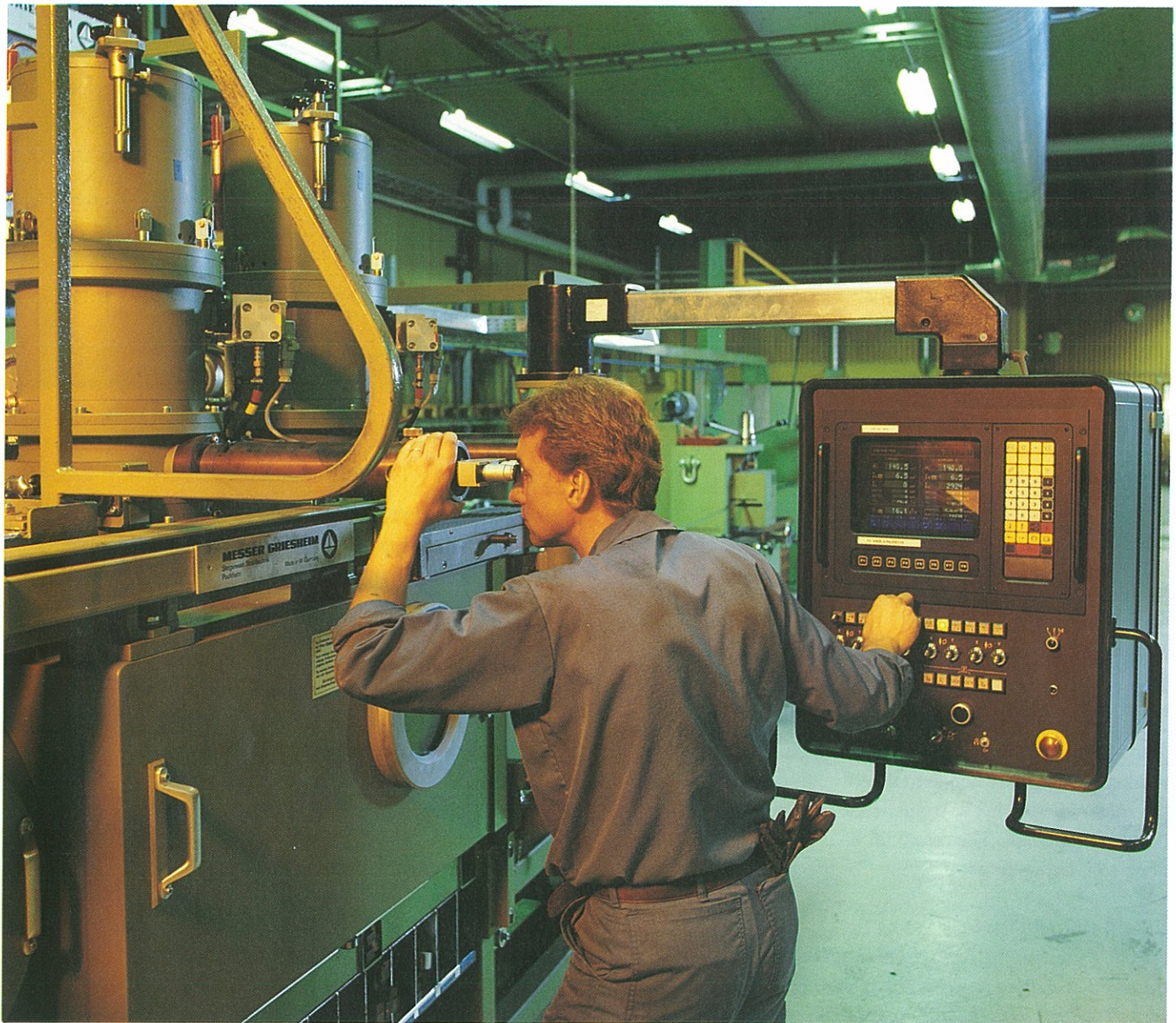
At Sandvik's product centre for metalcutting saws in Lidköping, bimetallic blades are welded under vacuum by an electron beam.
