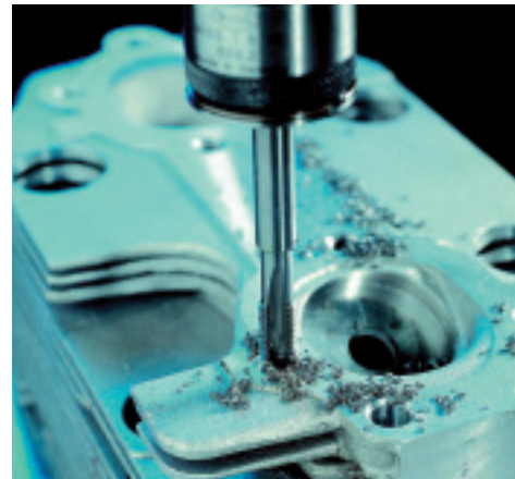
Prototyp within Sandvik CTT introduced a new type of threading taps for machining of stainless and high-alloy steel.
